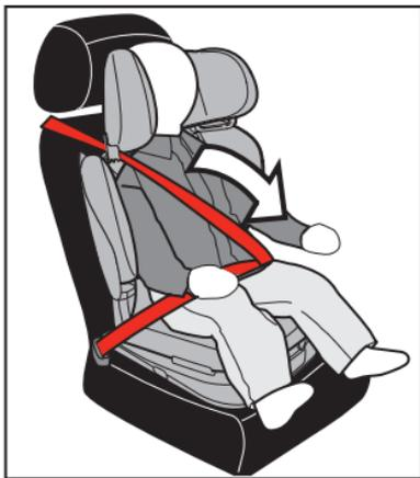
2. Fasten the vehicle seat belt, ensuring that it clicks in place. Position the two sections of the belt as shown in the picture.
